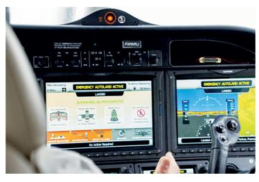
part of the G3000 integrated flight deck – and has been under development for the TBM since 2017 by the airplane systems department at Daher's Aircraft Division. This work included software implementation and an intensive flight test campaign that included two hundred automated landings.
