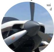
tzell Preside nt JJ Frigge. "And it has the Hartzell Top Prop 2,400 hour, 6 -year time between overhaul, and warranty until first overhaul," he added. The Hartzell Propeller Top Prop kit, HC-I3YF-1RF/F7498-1, is available for \$15,839 and includes a propeller, all-composite spinner assembly
